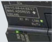
Communication and running state indicator, the PLC state can be seen easily.
