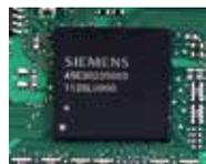
Siemens dedicated high speed chip is incorporated, with basic instruction execution time up to 0.15 μs;
