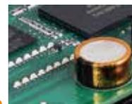
It is equipped with super capacitor, when the power is down, it still can guarantee the normal work of the clock
