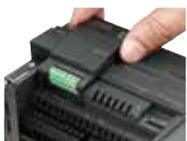
Signal board extension achieves accurate configuration, without occupying space in the electric control cabinet.
