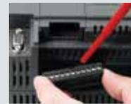
The input and output terminals of all modules are removable.
