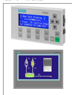
**Text Display unit:** The TD400C is a display device that can be connected to the CPU. Using the Text Display wizard, you can easily program your CPU to display text messages and other data pertaining to your application.
